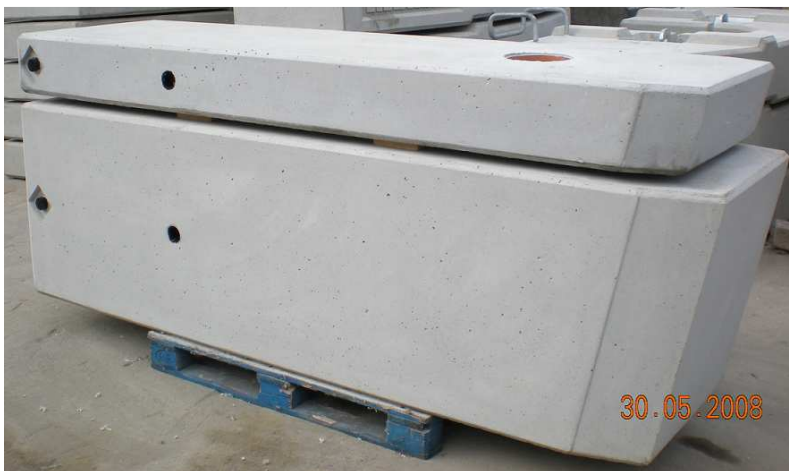
Picture: MDT City counter jib ballast CAU 3600 kg and CAV 1100 kg
